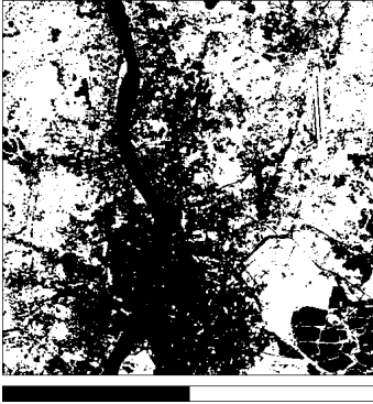
Fig. 42. Clustered image of Calcutta (using pixel gray value and average over its 3 \times 3 neighborhood)
